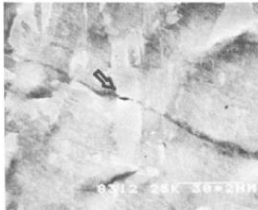
Micro-crack from plastic slip [6]
