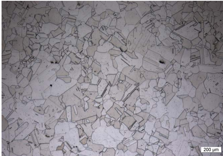
average grain size 52 μm
