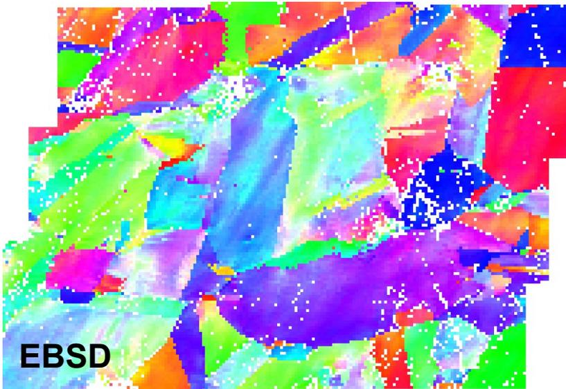
Damage factor include stress concentration and crystallographic orientation contributions.
