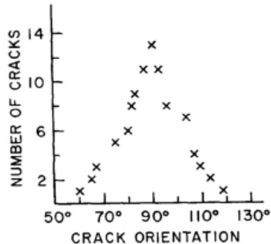
Frequency of micro-cracks relative to loading orientation [7]
