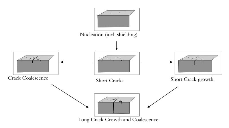
Different models for growth of small and long cracks
