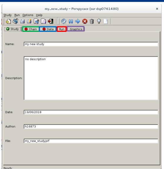
Chain tab: select the different modelling module and submodule and to link them
