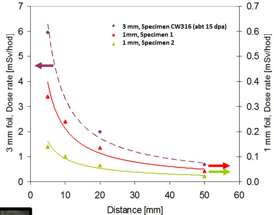
Figure: Dose rate from classical [3 mm] and currently developed [1 mm] TEM foils
