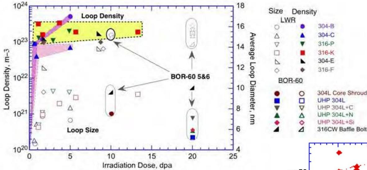
Results from the BOR-60 irradiation experiment with the data for austenitic stainless steels irradiated in a BWR [3]
