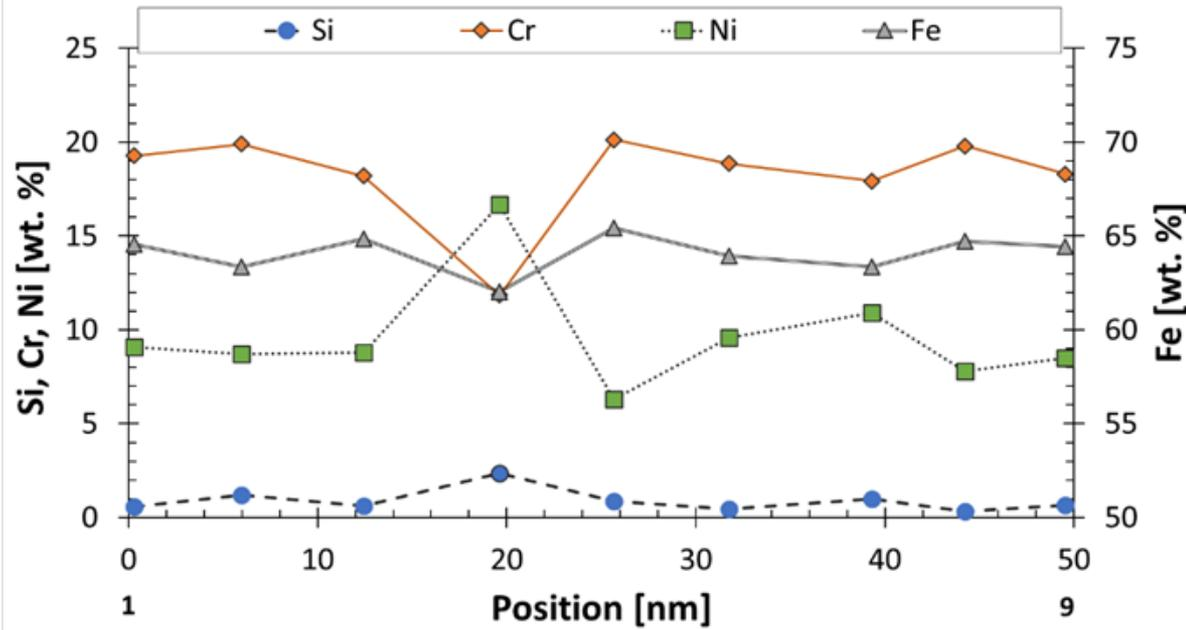
STEM EDS line scan across grain boundary; dashed line marks the position of grain boundary (GB) in the graph.
