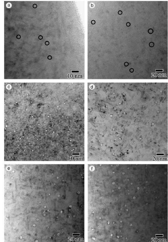
Examples are shown in (a) and (b) of the small cavities (encircled) present in a low density in the 1-mm bolt head position.
