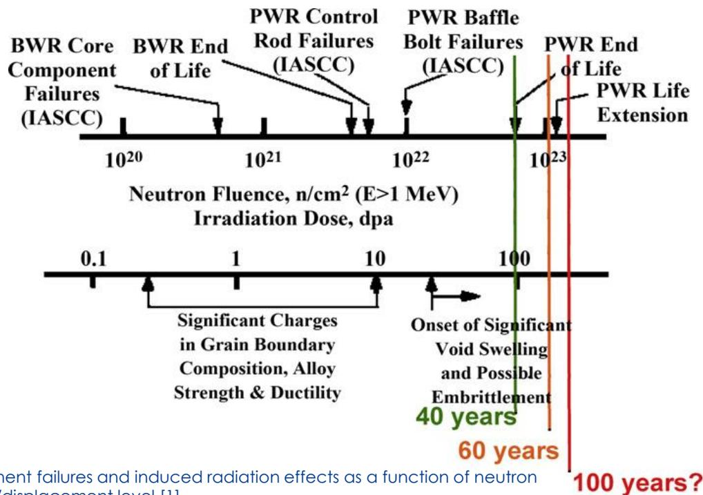
The 40-year lifetime fluence for reactor core internals in a BWR is  $4 \times 10^{22}$  n/cm<sup>2</sup> ( $E > 1$  MeV)
