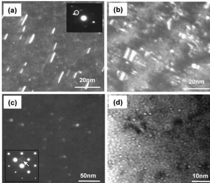
TEM images showing microstructural features observed in CW type 316 SSs PWR-irradiated to 53 dpa: (a) rel-rod dark field image of dislocation loops; (b) dark field image of dislocation loops and black dots; (c) dark field image of Ni<sub>3</sub>Si precipitates; and (d) defocused image of bubbles [Fukuya K, Fujii K, Nishioka M, Kitsunai Y. Evolution of microstructure and microchemistry in cold-worked 316 stainless steels under PWR irradiation. J Nucl Sci Technol. 2006;43:159–173.].
