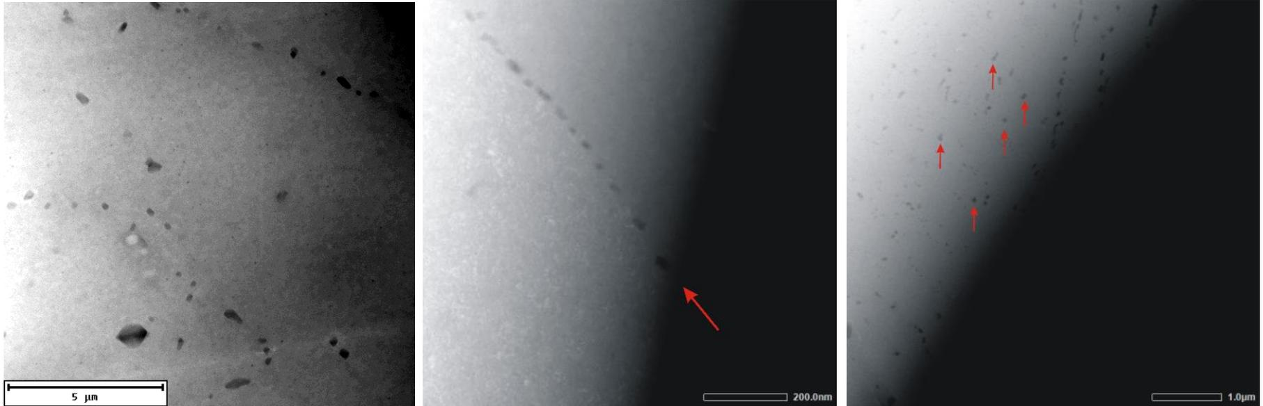
Ti-based precipitates distribution (right), decorating grain boundary of marked by red arrow (middle) and inside the austenitic grain (right), image taken in STEM mode using HAADF detector
