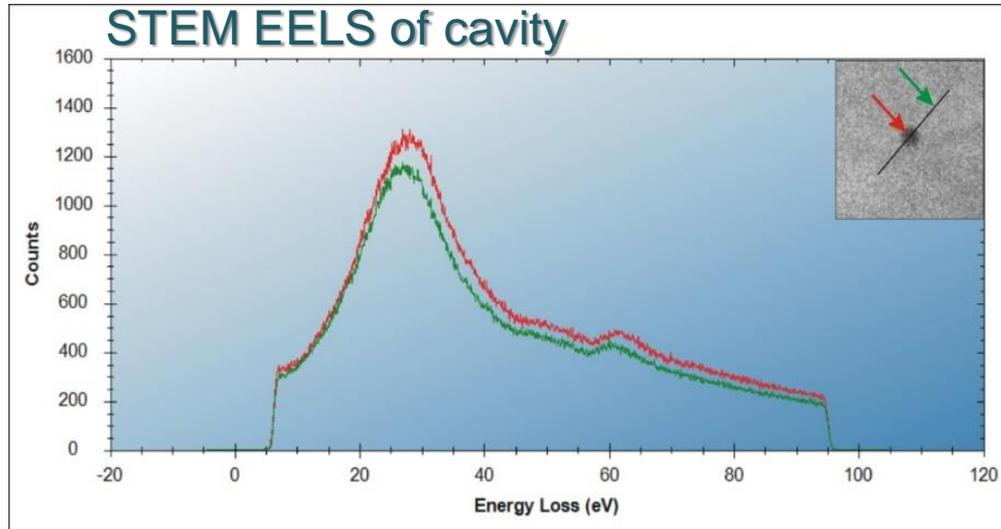
STEM EELS of cavity showing the scan line (black line) across the cavity where the EELS analysis was performed.
