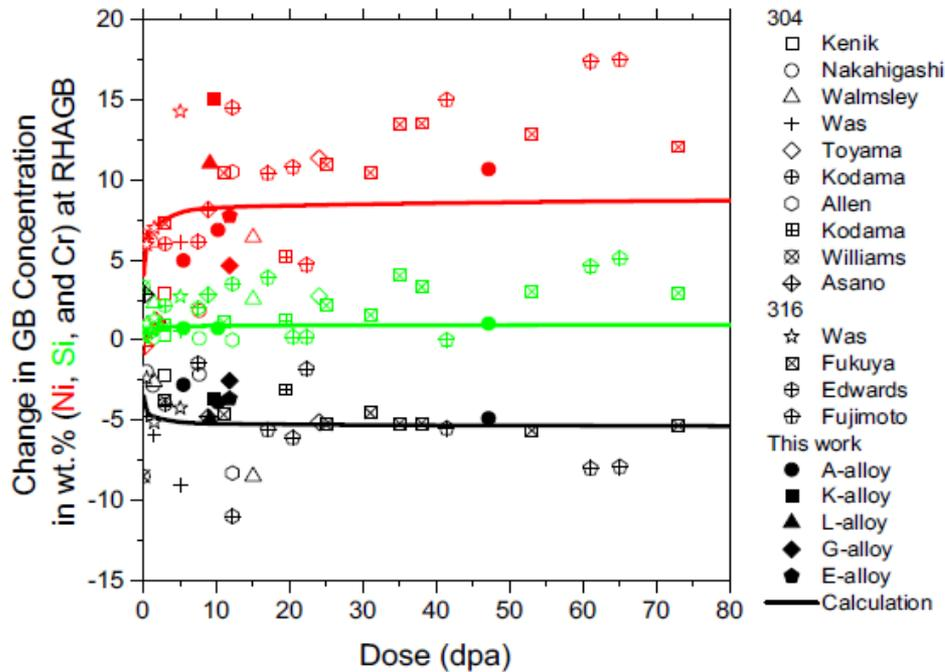
BOR-60 reactor at 320C for up to 47.1 dpa at a displacement rate of  $8 \times 10^{-7}$  dpa/s [7]
