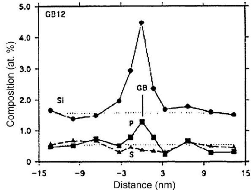
Conventional (V-shaped) grain boundary RIS profiles for a commercial purity 304 stainless steel neutron irradiated at 288 8C to 1.7 dpa [34]. Note depletion of iron and chromium at the boundary and enrichment of nickel, silicon and phosphorus[6]
