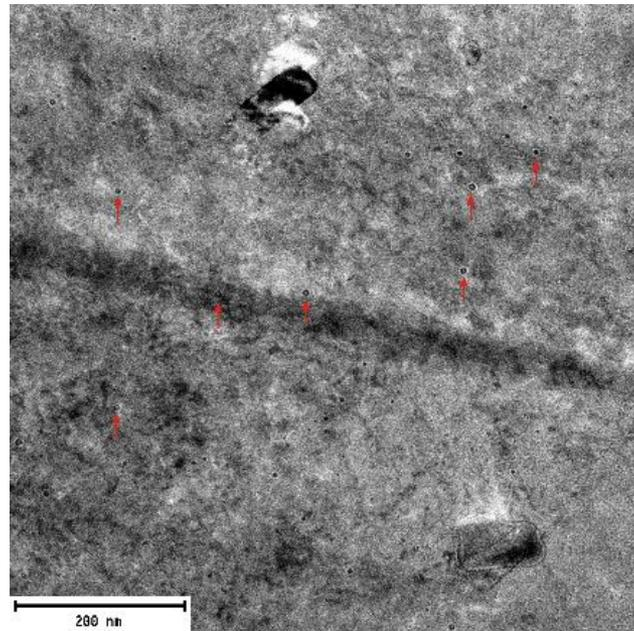
Cavities marking by red arrows: a) under-focused image, b) over-focused image
