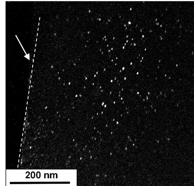
Figure 18. RIP in rel-rod DF micrograph (fast spectrum).
