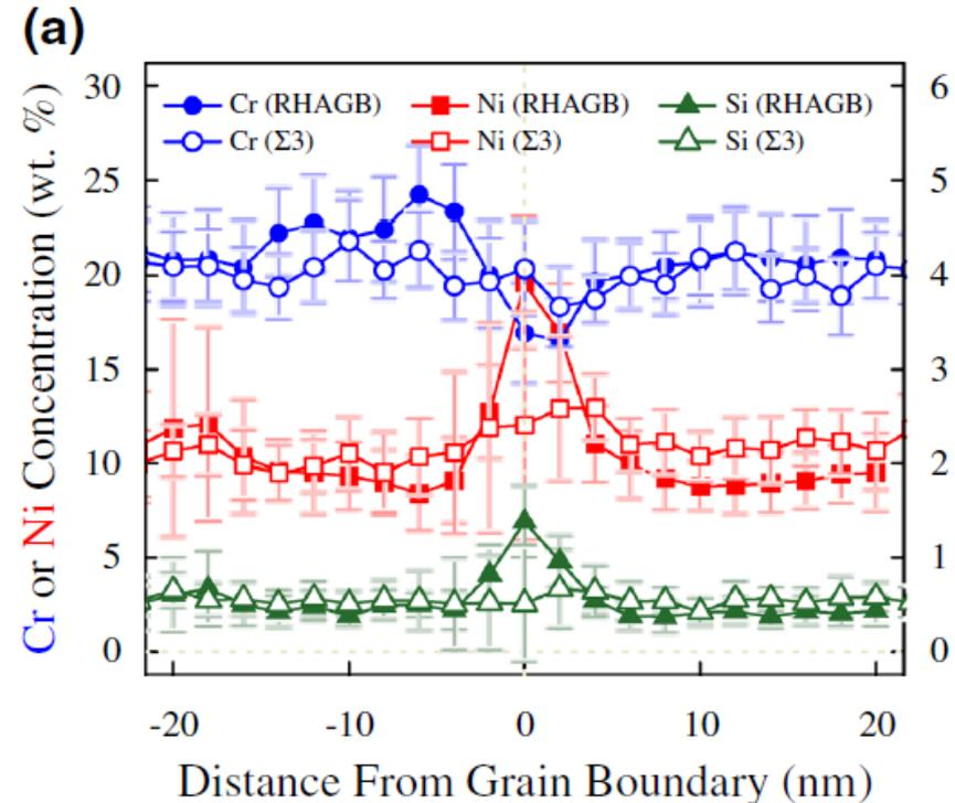
One-dimensional concentration profiles from random high-angle grain boundaries in the 47.1 dpa—irradiated specimen [7]
