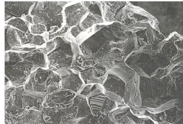
Intergranular fracture surface of a cracked bolt
