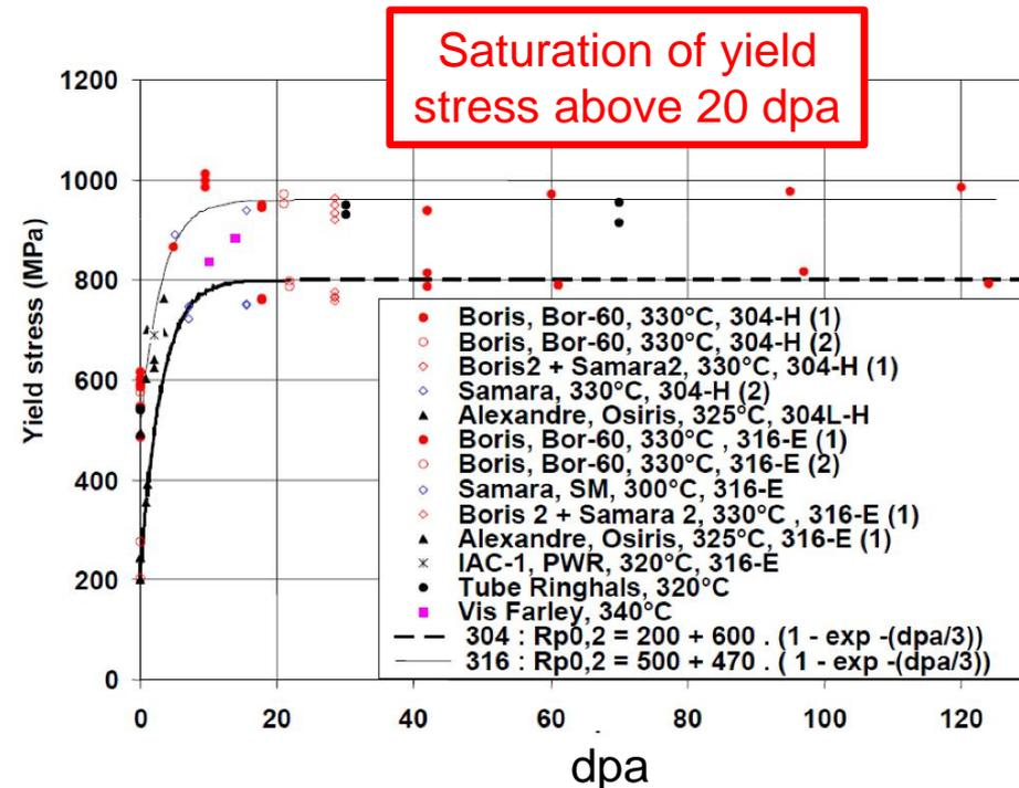
Saturation observed for  $R_{p0.2}$ ,  $R_m$  and  $e_U$  due to complex microstructural interplays
