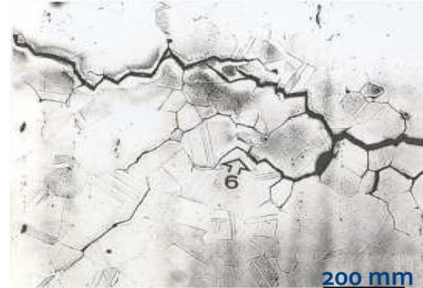
Intergranular aspect of a crack
