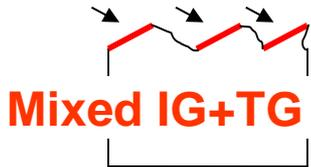
Fracture path inclined  $\sim 45^\circ$  to load axis
