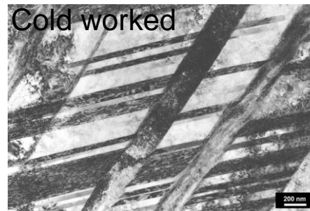
High density of deformation twins
