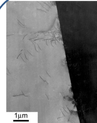
Solution annealed (SA) Low dislocations density (\rho_{ini} = \sim 10^{10} m^{-2})
