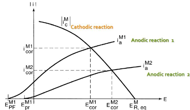
If the cathodic reaction rate is constant, free corrosion potential decreases when corrosion rate increase
