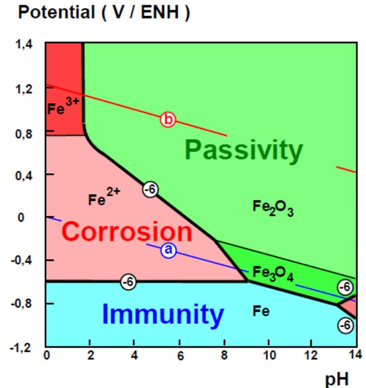
b) Corrosion diagram
