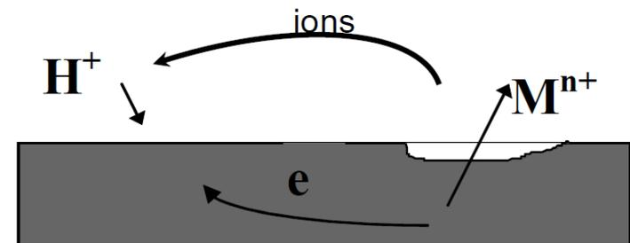
Aqueous corrosion (corrosion in LWRs)
