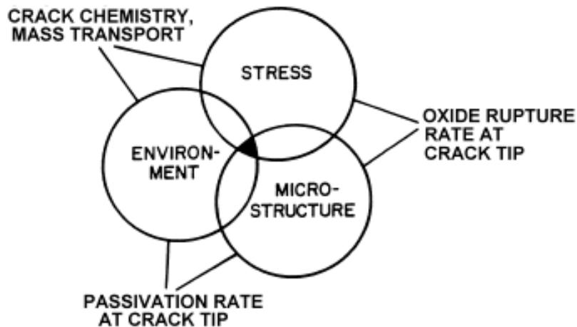
Crack depth vs. time =  $f(\text{Material, Stress, Environment})$
