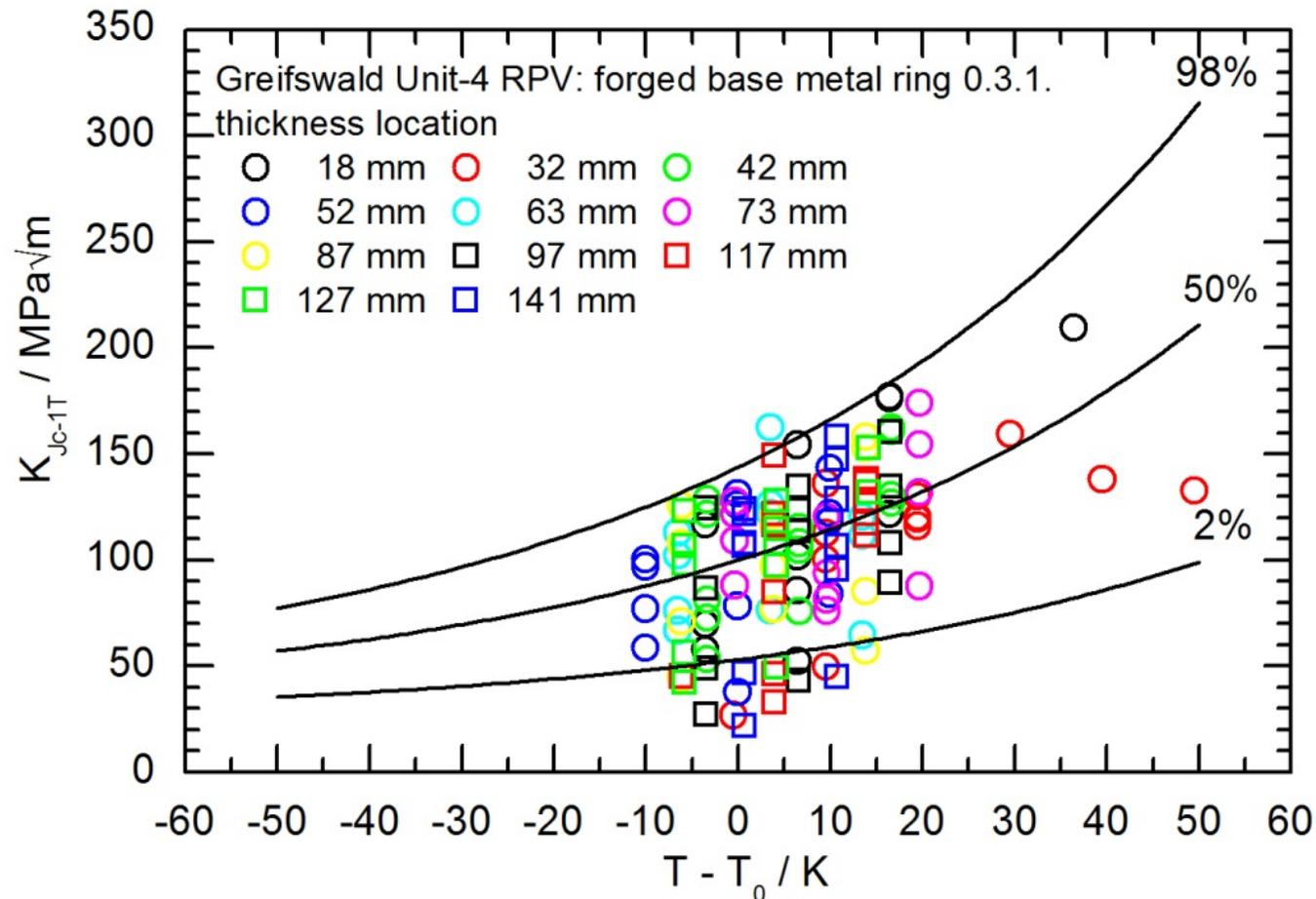
17 of 131  $K_{Jc-1T}$  values (13 %) lie below the fracture toughness curve for 2% fracture probability
