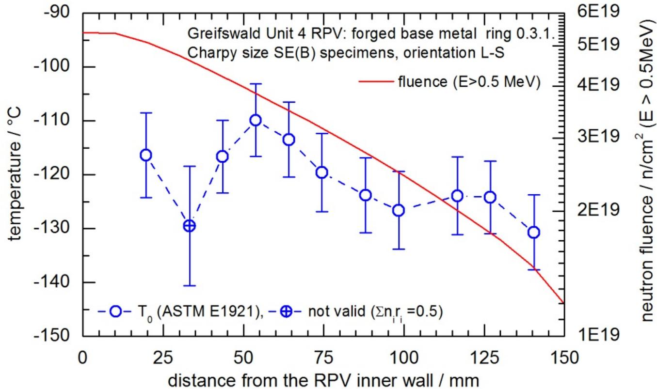
Progression of the MC reference temperature  $T_0$  through the thickness of the Greifswald Unit 4 forged base metal ring 0.3.1..
