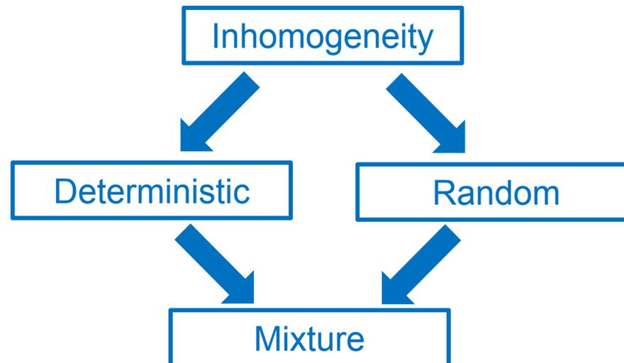
Deterministic inhomogeneity for example as a result of the location of the specimen in the forging can be accounted for. Random inhomogeneity is much more difficult to handle.
