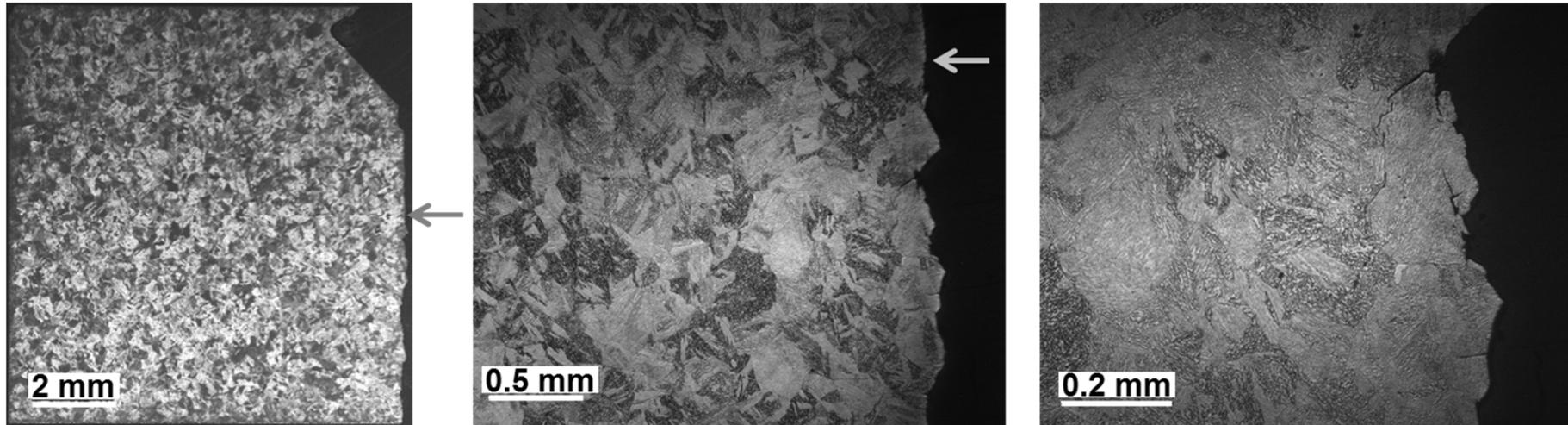
Microstructure of the forged base metal ring of the decommissioned RPV of Greifswald Unit 4.
