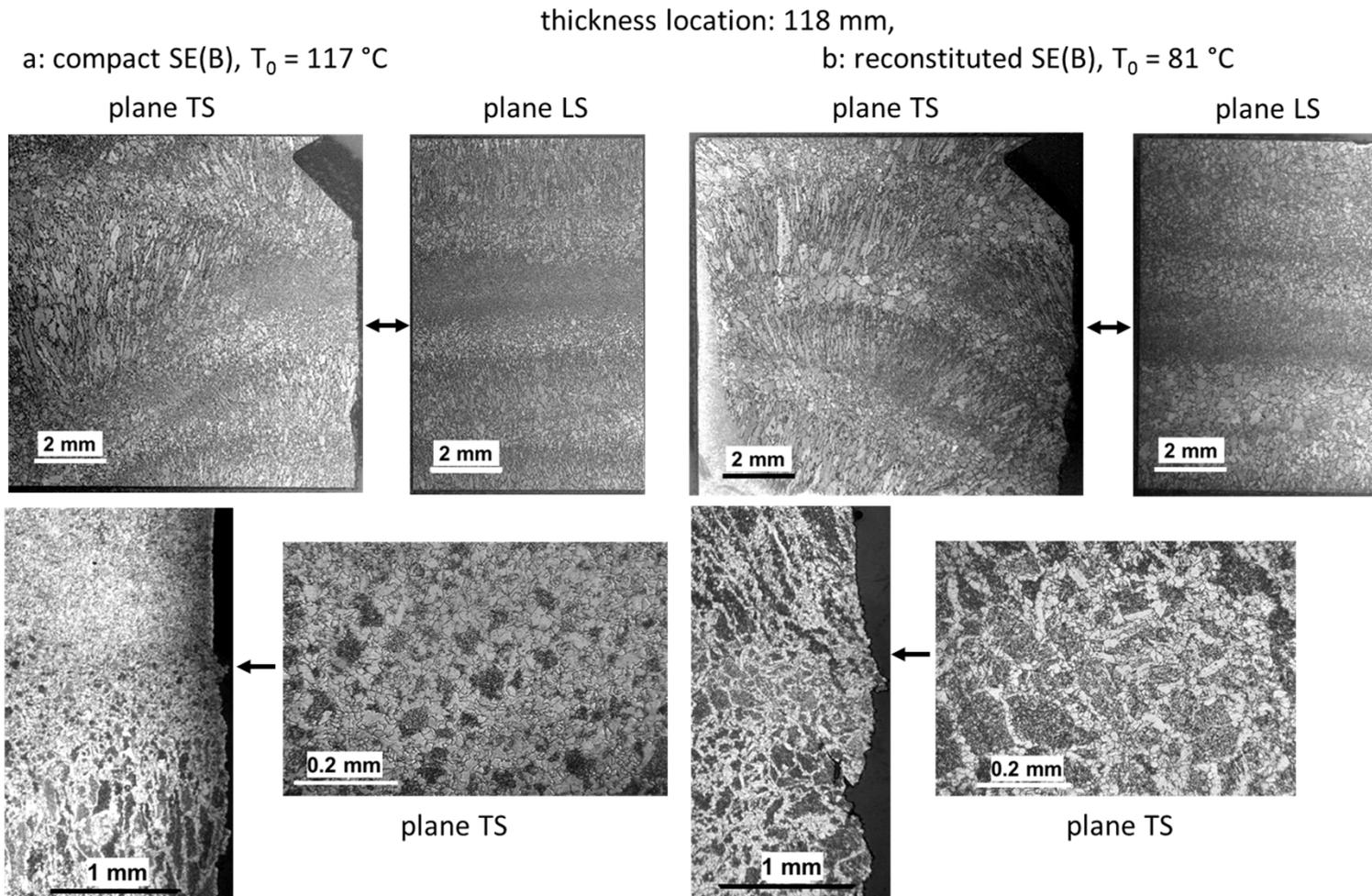
Metallographic sections of a compact (a) and reconstituted (b) T-S oriented SE(B) specimen from the thickness location 118 mm of the Unit 4 beltline multilayer welding seam (arrow marks the position of the crack tip).
