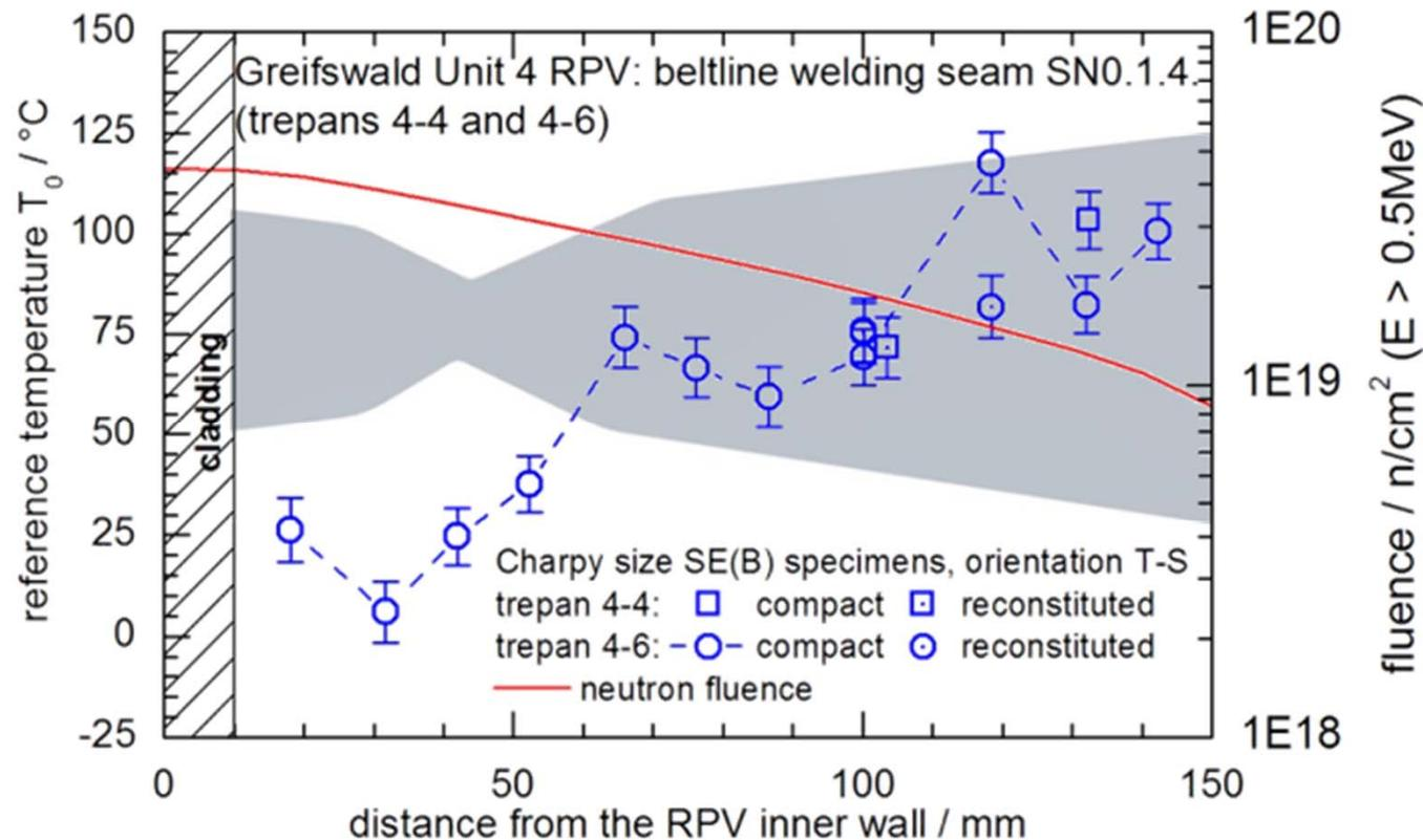
Progression of the reference temperature,  $T_0$ , through the thickness of the Greifswald Unit 4 beltline welding seam SN0.1.4 (trepan 4-4 and 4-6).
