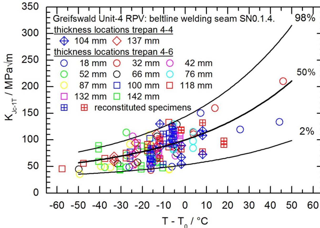
$K_{Jc-1T}$  values normalised with single-specimen-set  $T_0$  values and MCs of the Unit 4 welding seam SN0.1.4.: 11 out of 154  $K_{Jc-1T}$  values (7.1 %) are not enveloped by the 2 % and 98% tolerance curves
