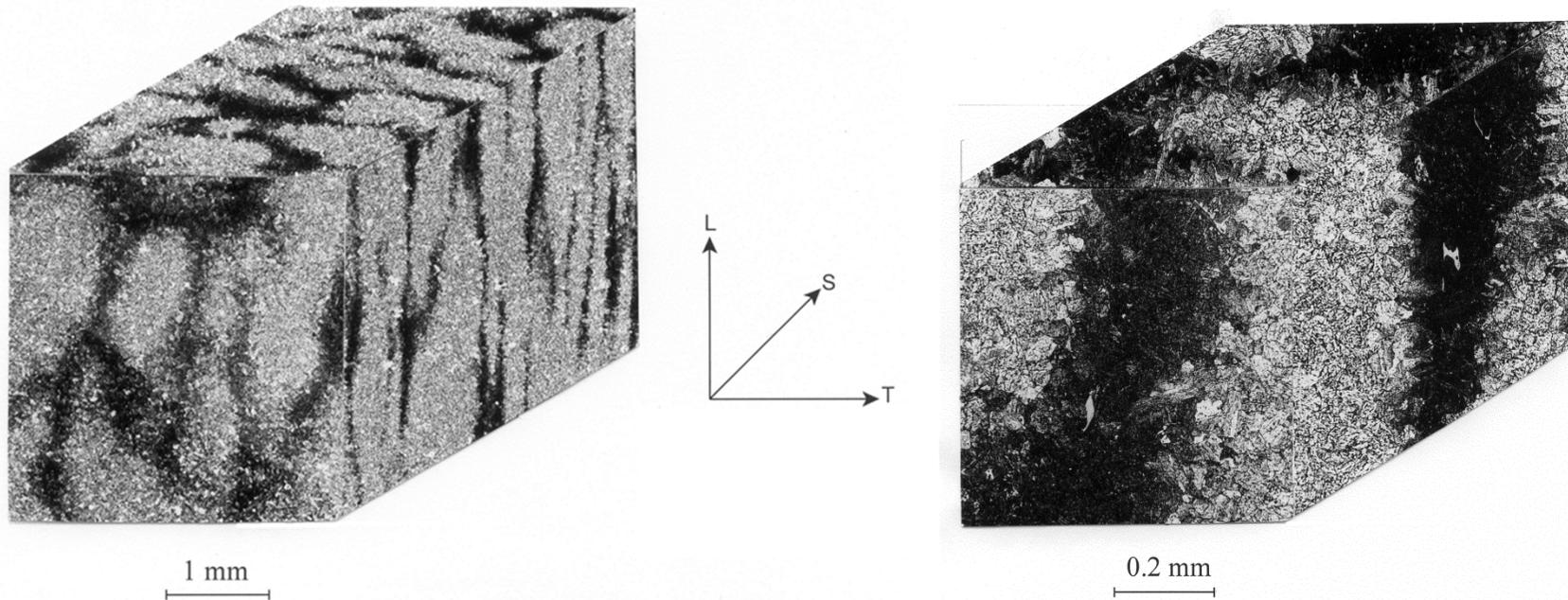
Microstructure of the rolled base metal plate of ASTM A533B Class 1 RPV steel (IAEA reference material JRQ).
