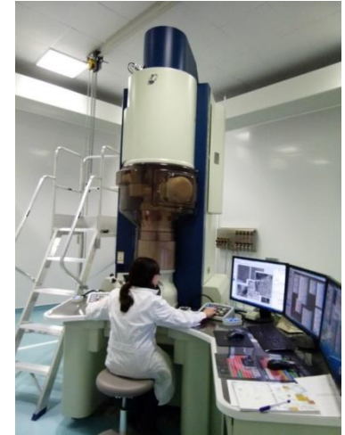
Jeol ARM 200F (double corrected, EELS, EDS, ADF, HAADF...)
