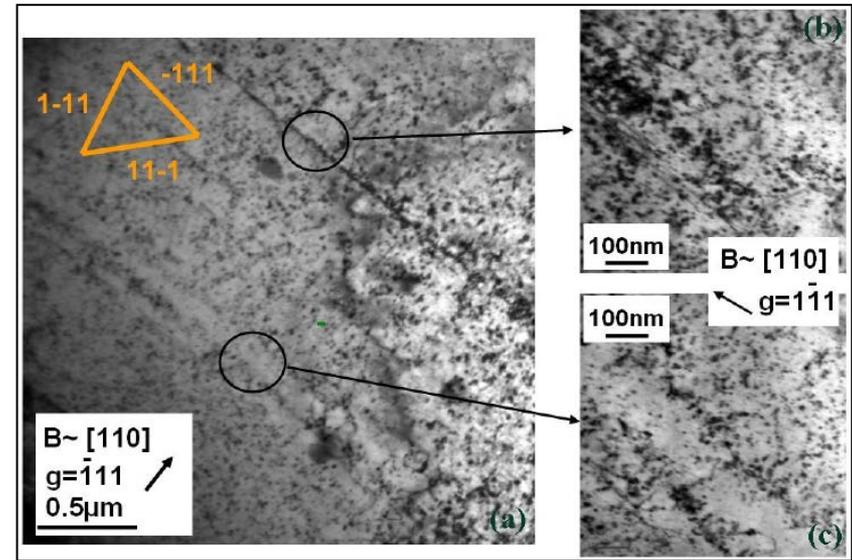
Initial propagation of shear band:
